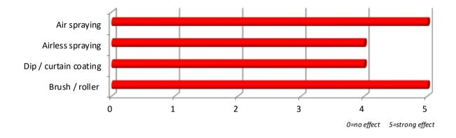
**UNID**<sup>®</sup>**FDAM 132 S** is medium to strong defoamer to be used in clear coatings as well suitable for pigmented coating systems. Due the chemical structure the product will not cause turbidity, but will give good air-release and macro defoaming properties. Also very well suited for PE primers remaining high clarity and transparency. The product is well suited for spraying applications.
